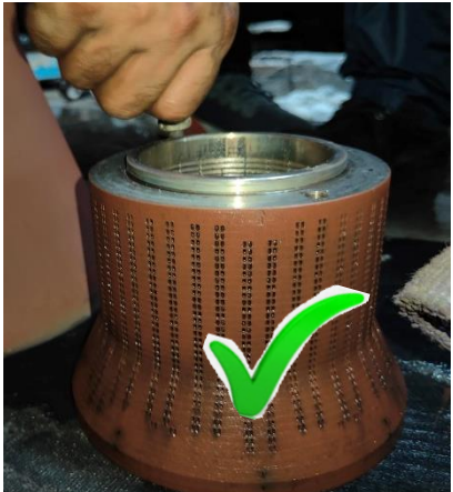
No damage to cage
